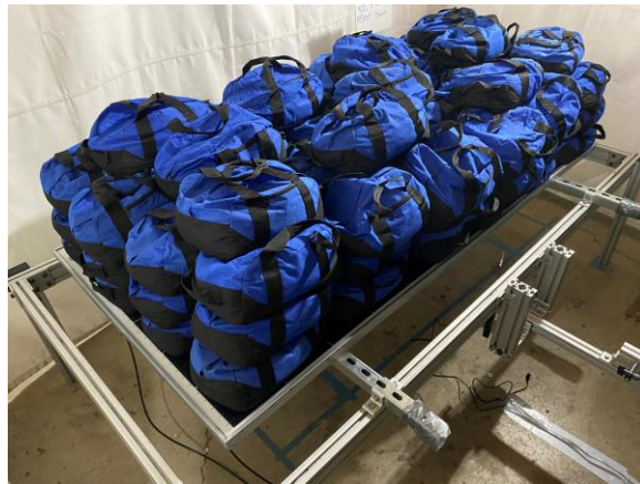
Steel frame undergoing UL and IEC testing
