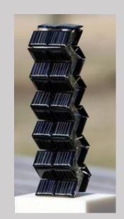
Stack prototype from MIT that demonstrated an increase in harvested electricity of 60%+ compared to a conventional array
