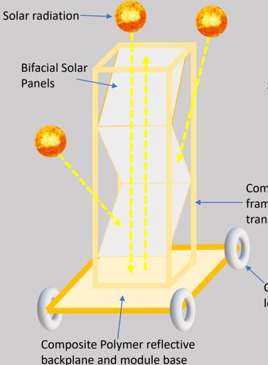
Portable system takes advantage of multiple angle of incidences of solar radiation as the sun transits while also maximizing bifacial panel functionality using a 90%+ reflective backplane.
