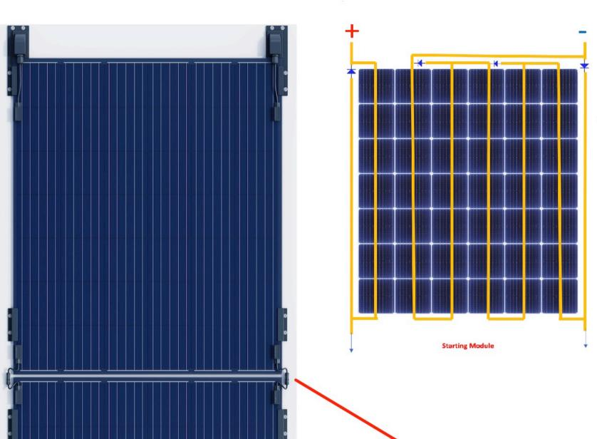
Cell configuration to have MC4 connectors at corners of module.
