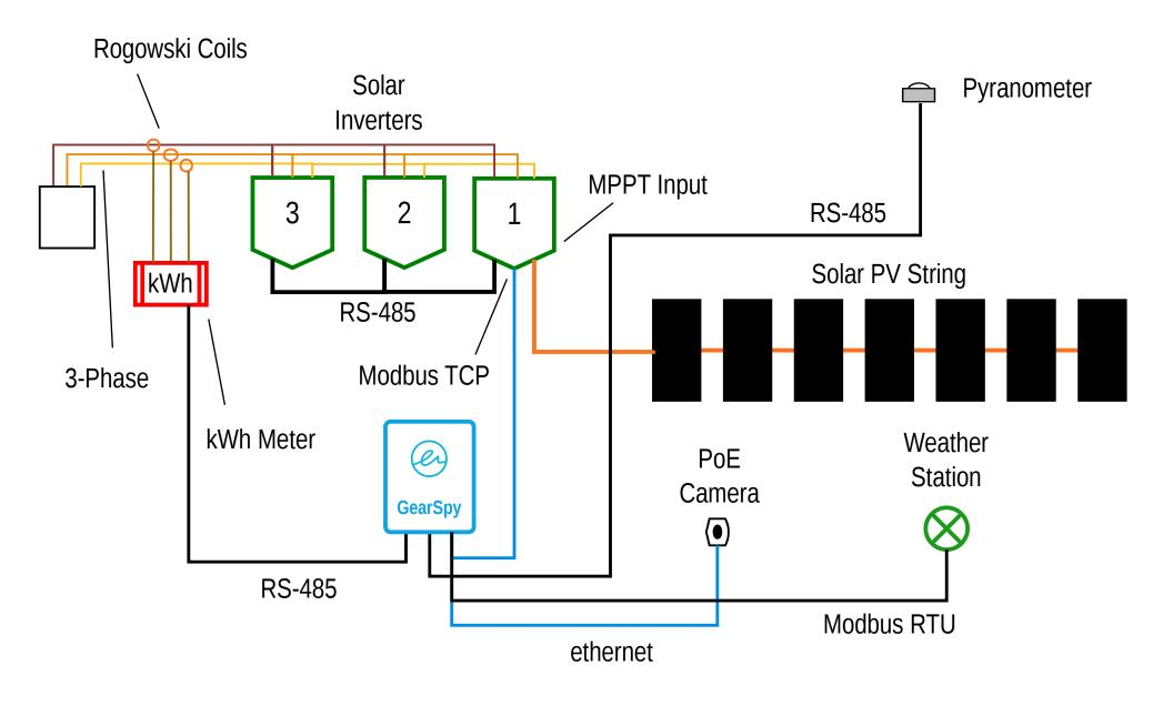
GearSpy is an open-source software able to run on an SBC to automatically identify C&I DER hardware and hardware configurations across multiple communication protocols and transport layers. Just Set it and Forget it to auto discover legacy and new DER across generations and topologies!
