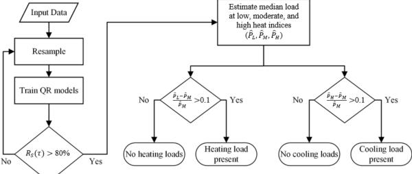
QRAM performs following steps to estimate load consumption under varying weather conditions:
