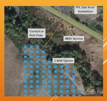
Installation #3 will be a private DG Power plant tied directly into the City distribution feeder lines. The install will allow continuation of tractor farming & agrivoltaic research.
