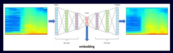
**Goal:** automated and scalable detection of incipient phenomena that can lead to future power disruptions. **How:** embeddings that enable the systematic comparison of synchrophasor-based spectrogram information.
