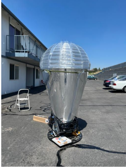
Fig.2 Prototype of the inflatable non-imaging non-tracking solar concentrator based CPVT system as an e-bike solar charging trailer
