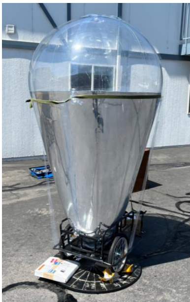
Fig.3 The inflatable non-imaging solar concentrator without domed flexible divergent Fresnel lens cover
