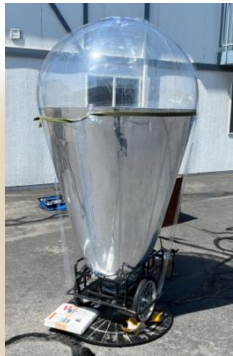
Fig.9 The inflatable non-imaging solar concentrator without domed flexible divergent Fresnel lens cover CPV on a e-bike trailer
