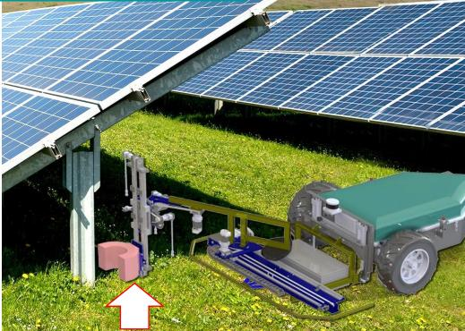
Global Neighbor will work with Renu Robotics and Rixan Automation to develop a robotic arm, equipped with proprietary Directed Energy Flora Control technology, to **autonomously control vegetation around mounting posts, without chemicals**
