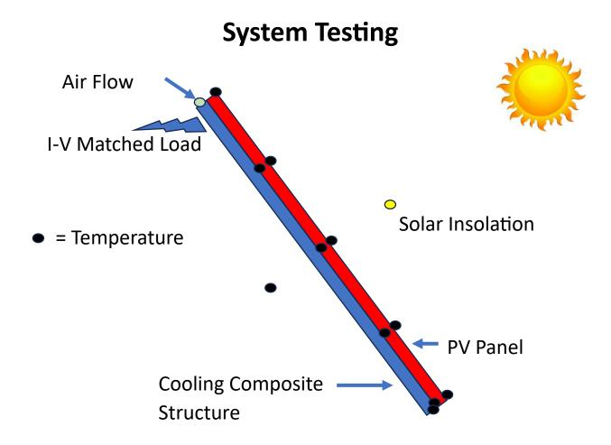
So as to have data on the cooled PV system relative to a non-cooled PV panel, we request that the above test layout also be performed on a matched PV panel that does not have the cooling system.
