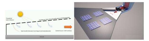
Heat from transpired collectors provide the driving force and can be coupled with PV arrays in a PVT configuration to recover the thermal energy and produce more power.
