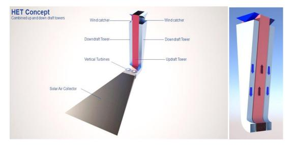
The Solar Thermal Power Tower includes transpired solar air collectors, solar updraft tower, wind downdraft tower, Venturi or shrouded chamber for turbines, phase change material (PCM) thermal storage and integration of PV with recovery of wasted PV heat. A recent objective is to utilize the towers in fire prone areas and situated as firebreaks. The towers can also attract lightning and store it in ground as thermal energy.
