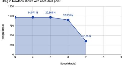
Viable 200ft Barge Operating Speeds & Weights Drag in Newtons shown with each data point
