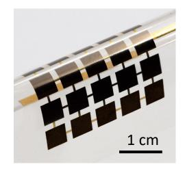
Material processes are liquid solution-based and offer an attractive price point for both rigid and flexible cells
