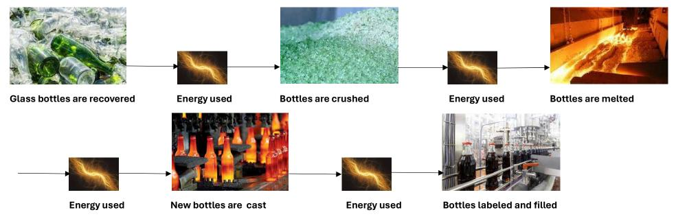
As recovered glass bottles are recovered, then crushed, melted, cast, filled, and labeled, energy is used at each step.
