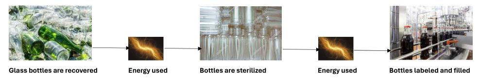
Glass bottles are cleaned and sterilized and then filled and labeled using far less energy and materials in the reuse process.
