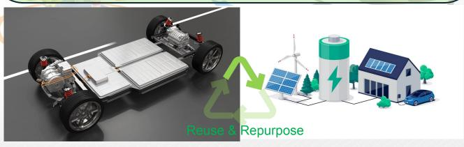
In its second life, a fully charged EV battery can consistently power a household for 2-6 days, ensuring grid independence.
