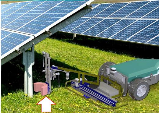
Global Neighbor is working with Renu Robotics and Rixan Automation to develop a robotic arm, equipped with proprietary Directed Energy Flora Control technology, to **autonomously control vegetation around mounting posts, without chemicals**
