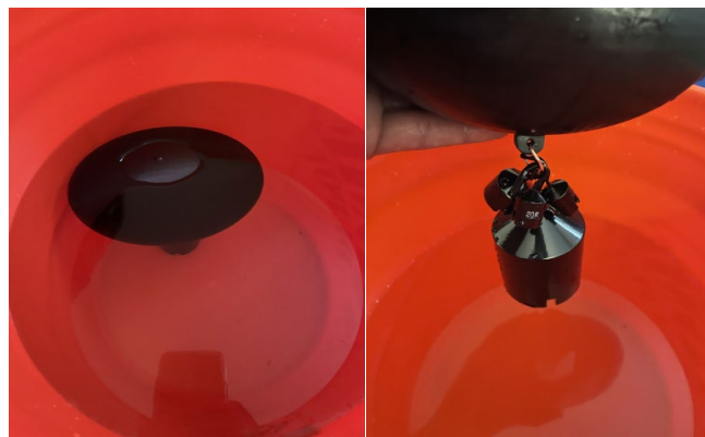
Figure 10 Buoy completely submerged and stationary (left), Buoy with weights attached (right)
