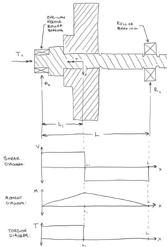
**Figure 13:** Shear, moment, and torsion diagrams for the pinion shaft.
