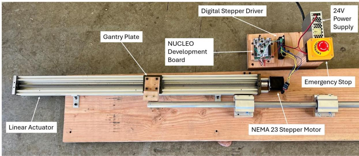
**Figure 12:** Electronics driving the linear actuator.
