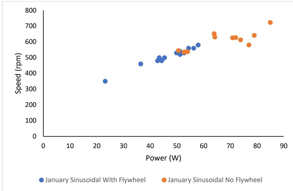
**Figure 34:** Power vs speed graph for January sinusoidal waveforms with and without flywheel measured with a 10 Ohm resistive load.
