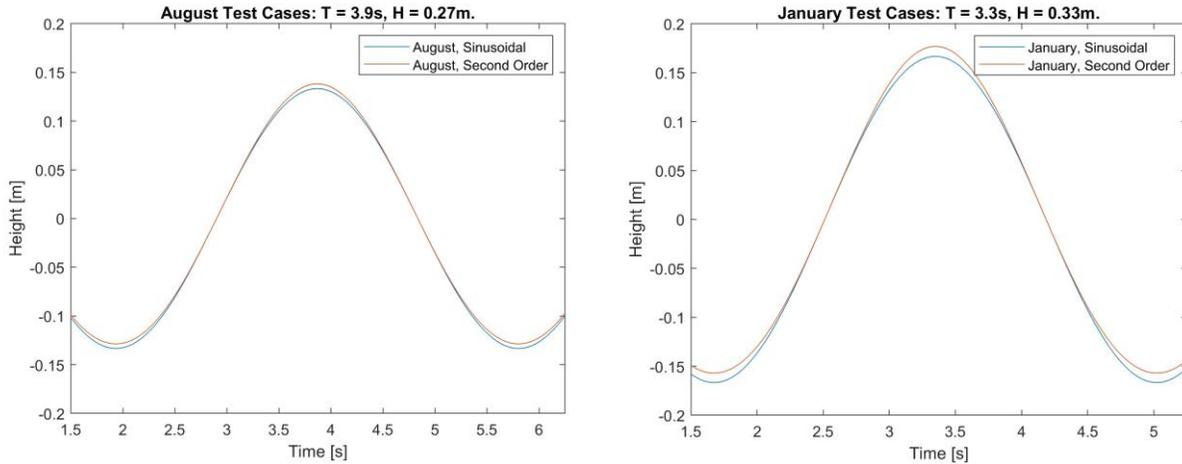
**Figure 21:** Linear (sinusoidal) and second order wave heights, overlaid.
