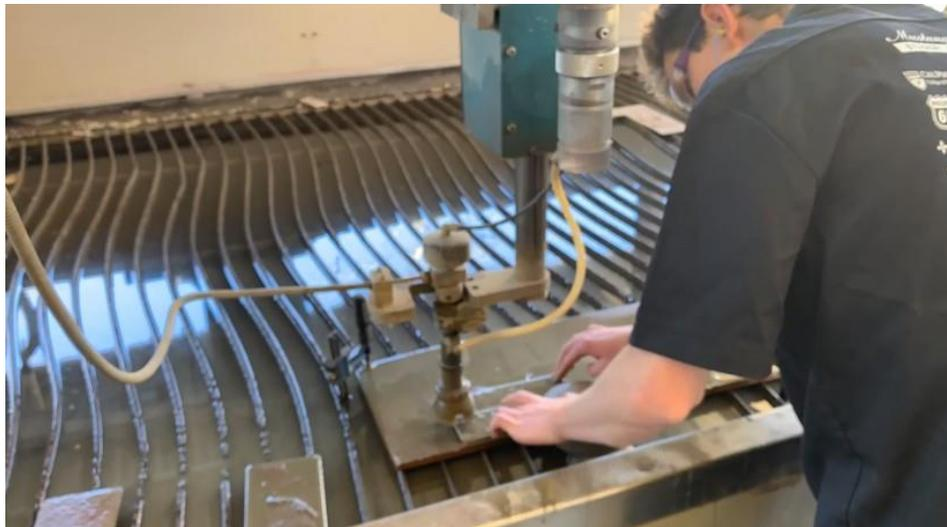
**Figure 24:** Mechanical team member Brendan secures an aluminum plate to cut out the rack plates on the Cal Poly waterjet.
