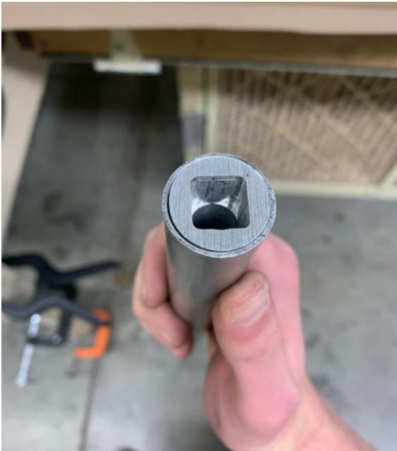
**Figure 22:** Machined spacer to connect the u-joint to buoy pole.
