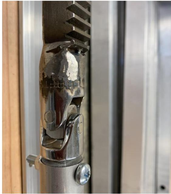
**Figure 23:** Welded u-joint to rack, buoy pole and u-joint connected with the spacer in Figure 22.
