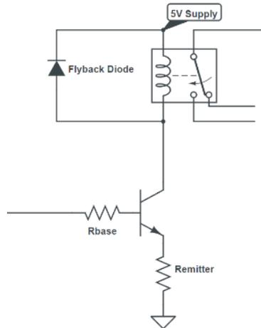
**Figure 11:** Current amplification circuit using a BJT.
