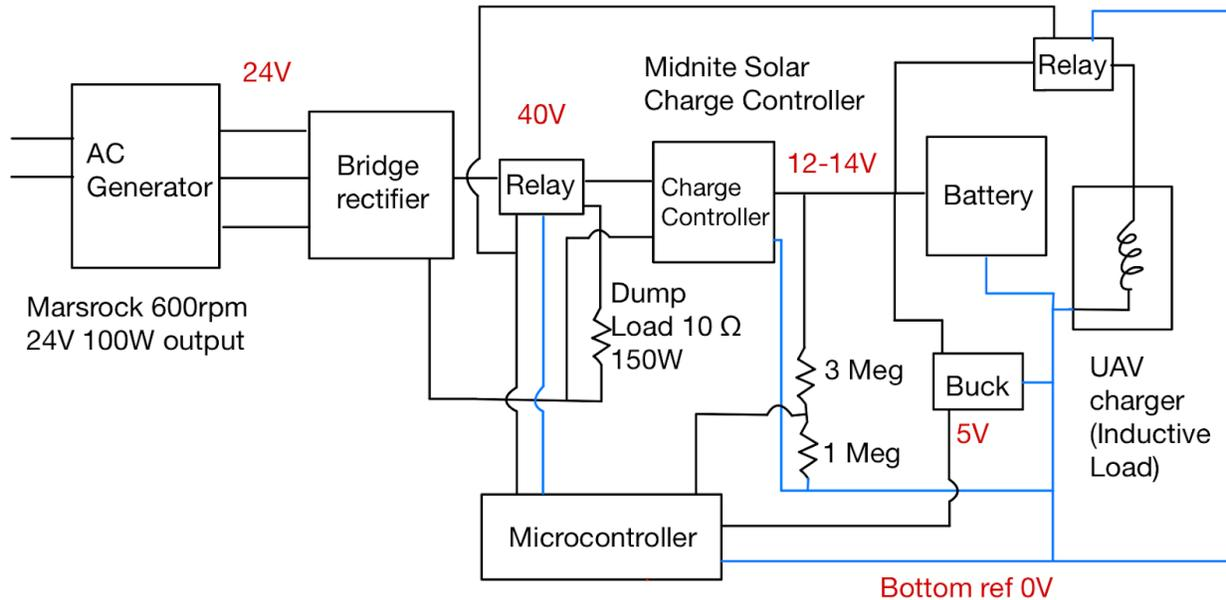
**Figure 10:** High level system schematic.
