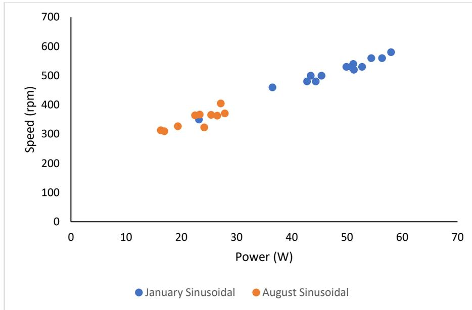
**Figure 35:** Power vs speed graph comparing January sinusoidal waveforms with August sinusoidal waveforms measured with a 10 Ohm resistive load.
