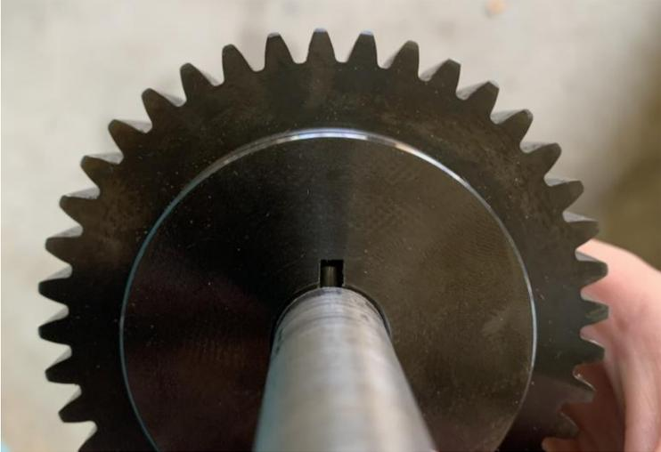
**Figure 25:** Broached keyway in the pinion, with shaft and key in place.
