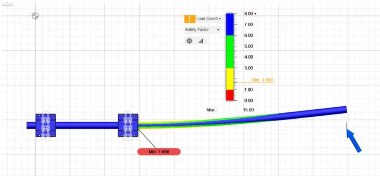
**Figure 14:** FEA for 60 degree load angle respectively
