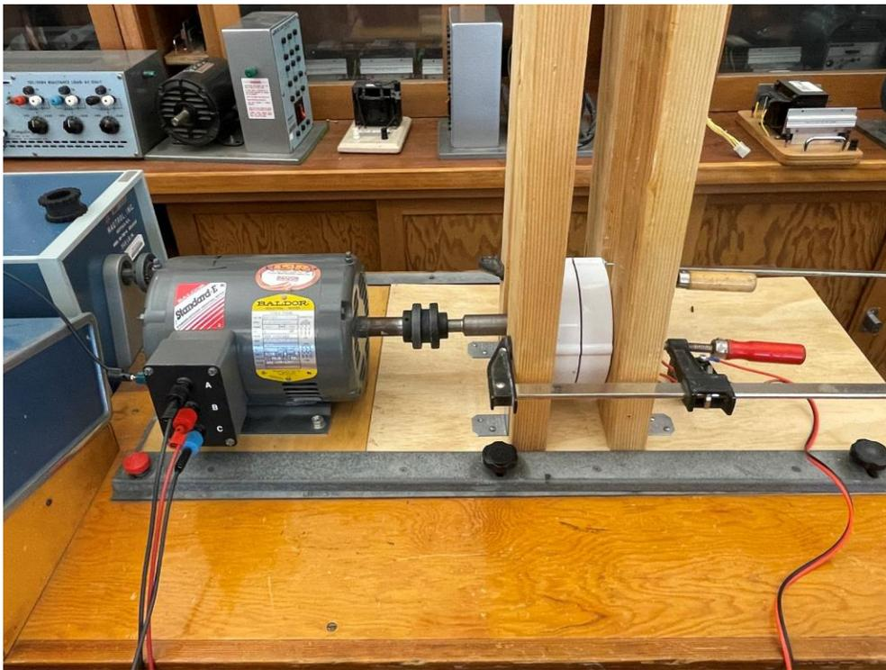
**Figure 32:** Motor and generator testing setup.
