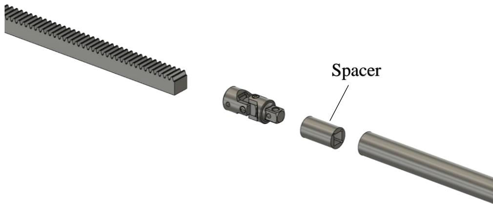
**Figure 8:** Rack to buoy pole connection exploded view.
