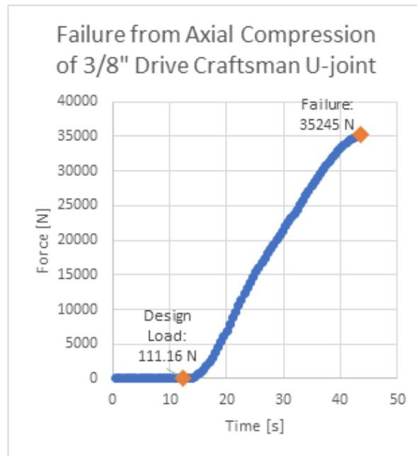
**Figure 29:** Ametek test results.
