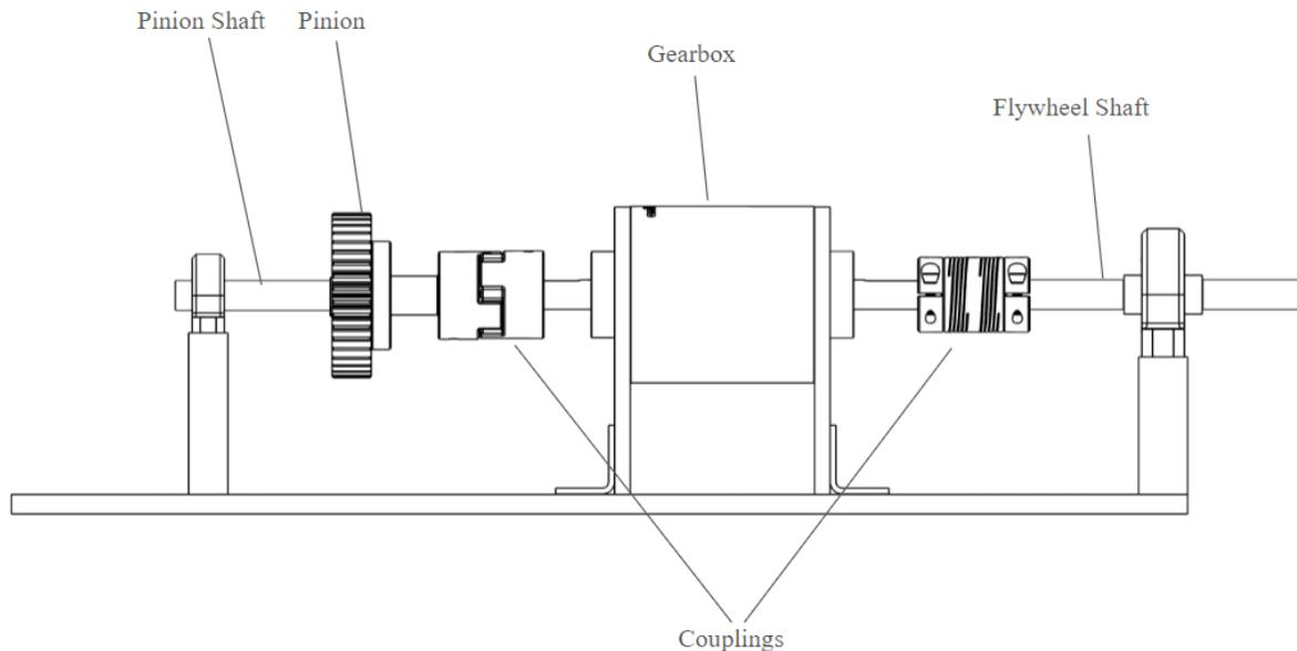
**Figure 9:** Side view of rotational mechanical subsystem.
