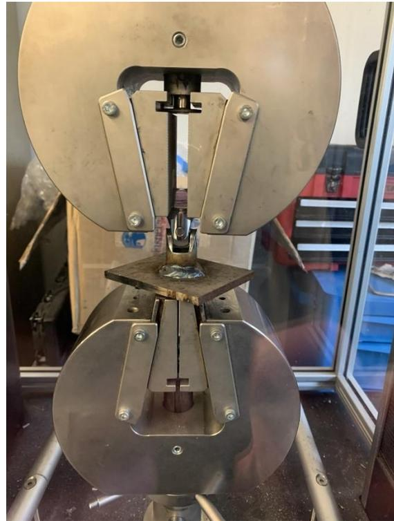
**Figure 28:** Male end of u-joint in testing vise, welded end compressing into bottom vise.
