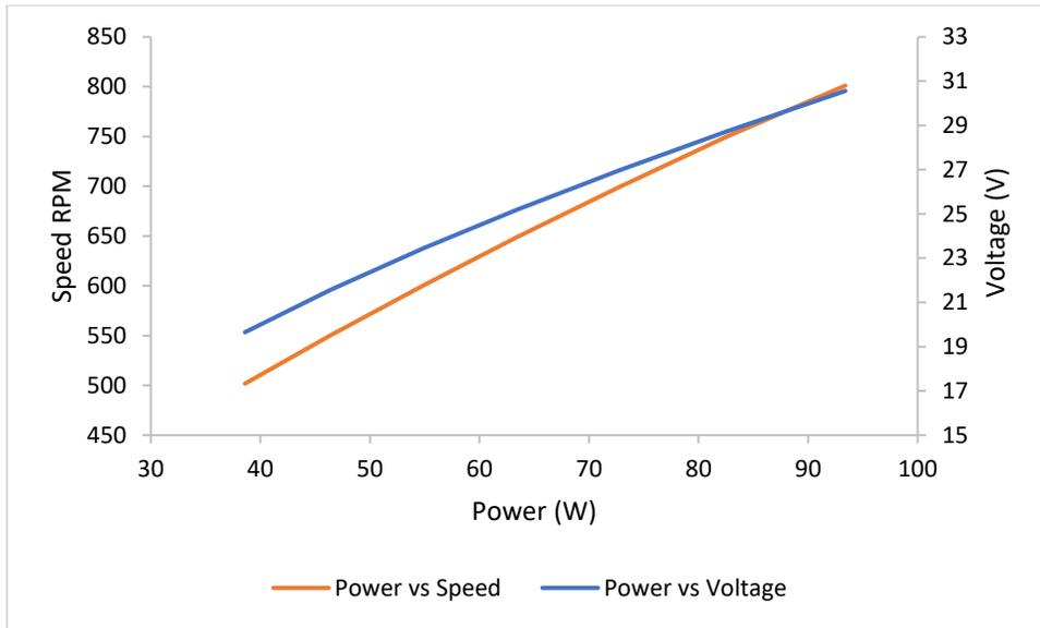
**Figure 31:** Generator characteristics for a constant load.
