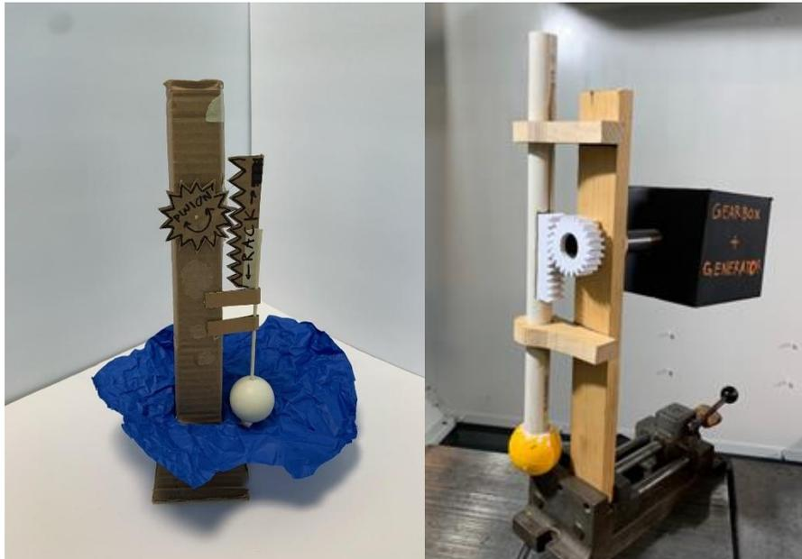
**Figure 18:** Progression of rack-and-pinion prototypes.
