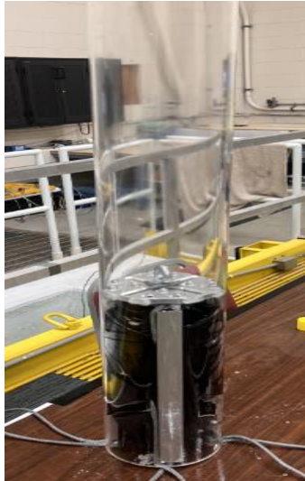
Figure 4.2: Ballast System Collapsed in Mock Sonobuoy
