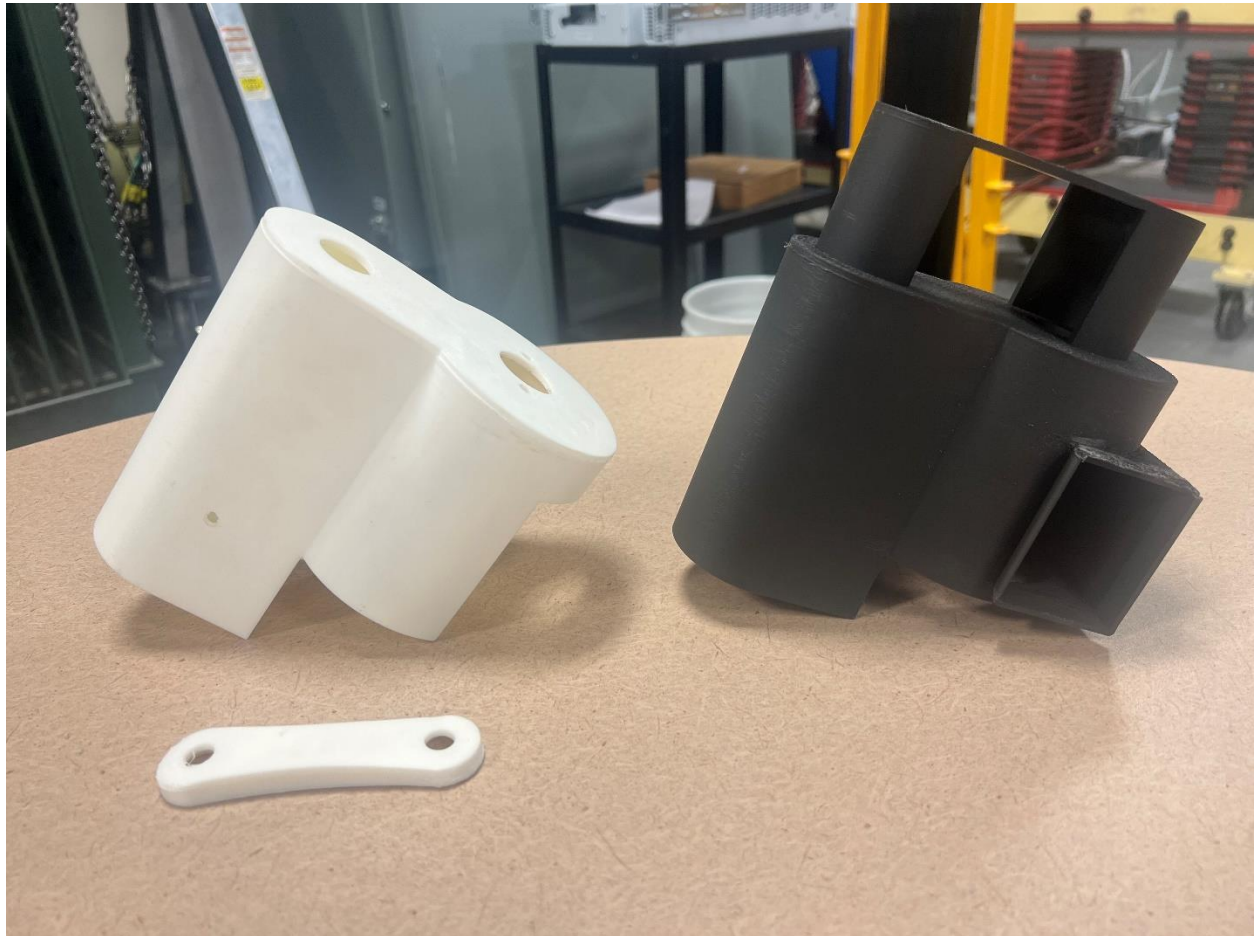
Figure 15: Previous (Left) and Current (Right) Motor Mounts
