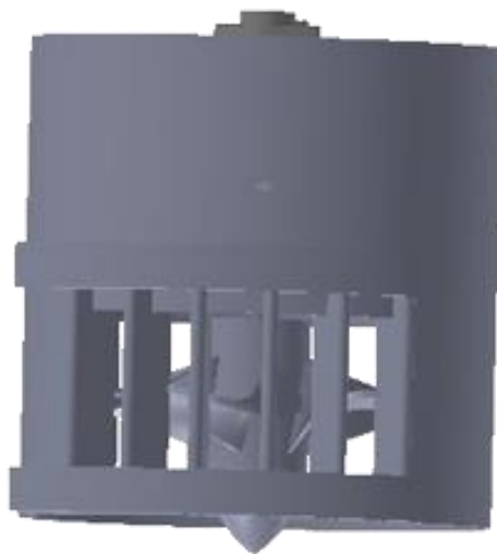
Figure 8: A design modification made to have guiding vanes level with rotor blades.
