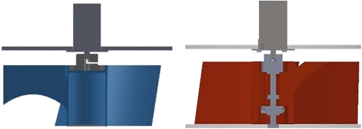
Figure 11: Design with generator directly connected to rotor hub (left). Design with a shaft and bearings connecting rotor and generator (right).
