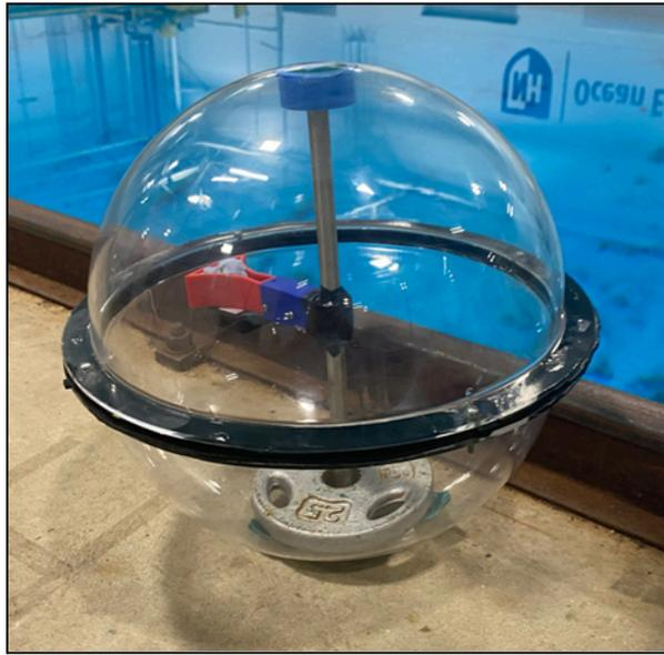
*Figure 18: First prototype of Drift-RMT*
