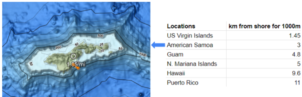
Figure 6: Distance from the shore to 1000 meters in depth using the National Oceanic and Atmospheric Administration (NOAA) mapping tools [7, 36-39]
