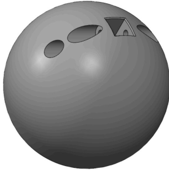
Figure 27: The buoyant sphere which supplies an upward force on the shaft. Constructed from ABS plastic and contains holes in order to mount itself to the shaft.
