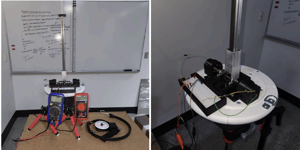
Figure 52: Photos of WEC power generation Test Setup
