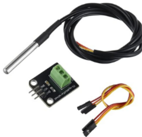
Figure 31: DS18B20 Temperature Sensor
