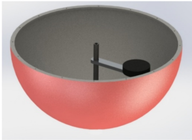
Figure 2: Design Concept of WEC: A Hemisphere with Rotating Pendulum, Source: 1
