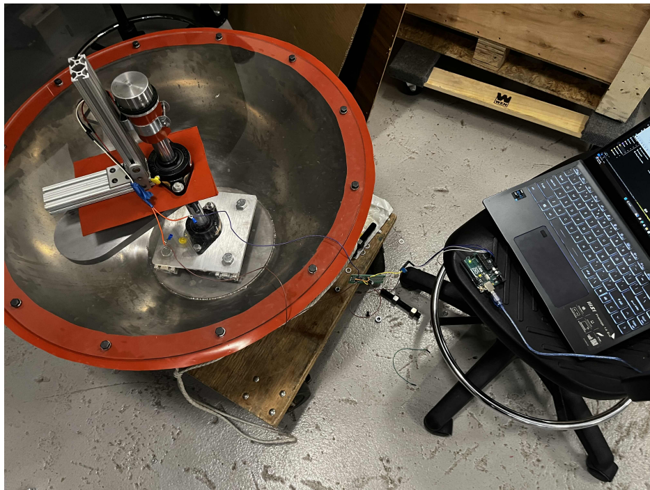
Figure 51: AC Generator and Pendulum Device
