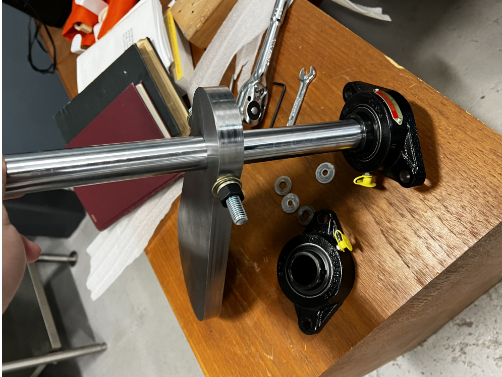
Figure 39: Actual Fabricated Pendulum and Shaft
