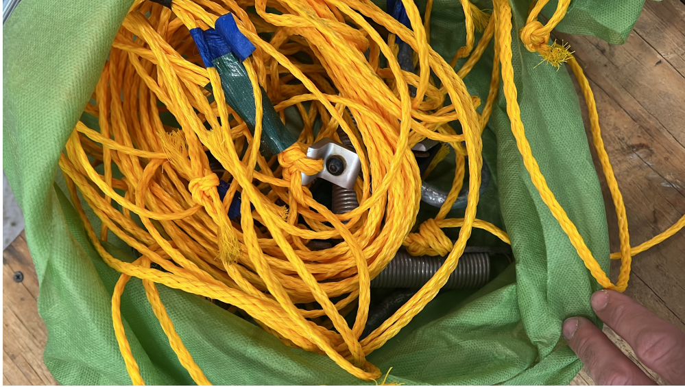
Figure 56: Tether Mooring Lines for Easy Fixation and Deployment, anchored to 100 lbs on the bottom of the Wave Tank
