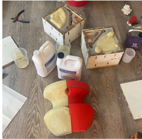
Figure 3.2 Mold Casting the Hull Shapes
