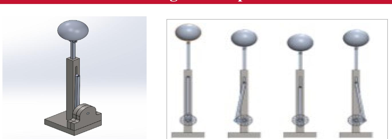
A buoyant surface component couples the wave motion via a sliding piston to an underwater four-bar crank mechanism driving a generator's rotating shaft. Critical features include a dual-crank, a flywheel providing inertial energy storage for consistent generator operation, and a gearbox boosting  $\frac{8}{3}$  is a the input speed to the optimal generator rpm.
