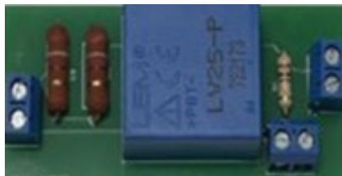
Fig.5 LV25-P Voltage Sensor PCB
