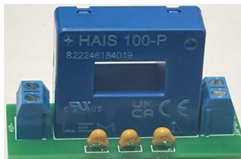
Fig.7 Designed Current Sensor fabricated on a PCB
