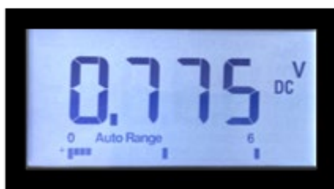
Fig.6 Voltage Sensor reading with 25V input
