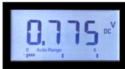
Fig.6 Voltage Sensor reading with 25V input
