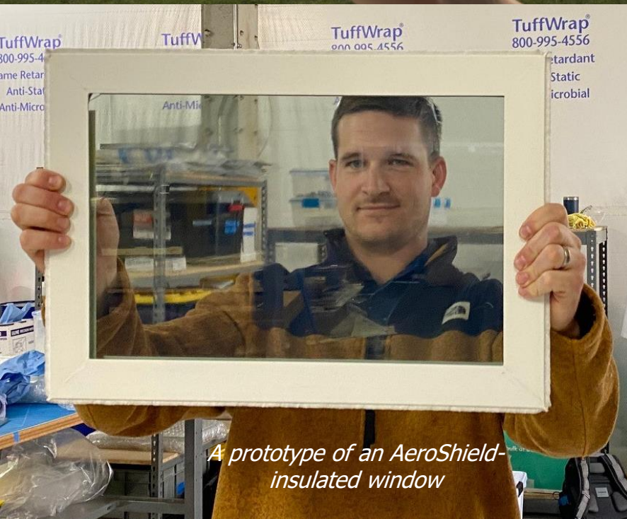
A sample showing AeroShield's record-breaking clarity
