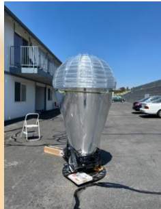
Fig.4 Prototype of the inflatable non-imaging non-tracking solar concentrator based CPV system on a e-bike trailer
