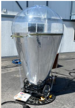
Fig.9 The inflatable non-imaging solar concentrator without domed flexible divergent Fresnel lens cover CPV on a e-bike trailer
