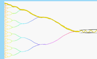
Fiber Optic Concentration Network
