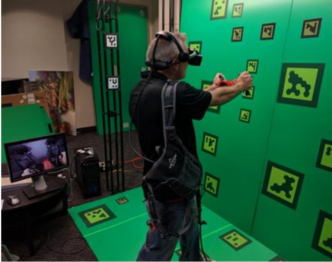
This image shows a trainee using a real fire hose in a virtual environment. The screen shows what the trainee sees, their real hands and the fire hose.
