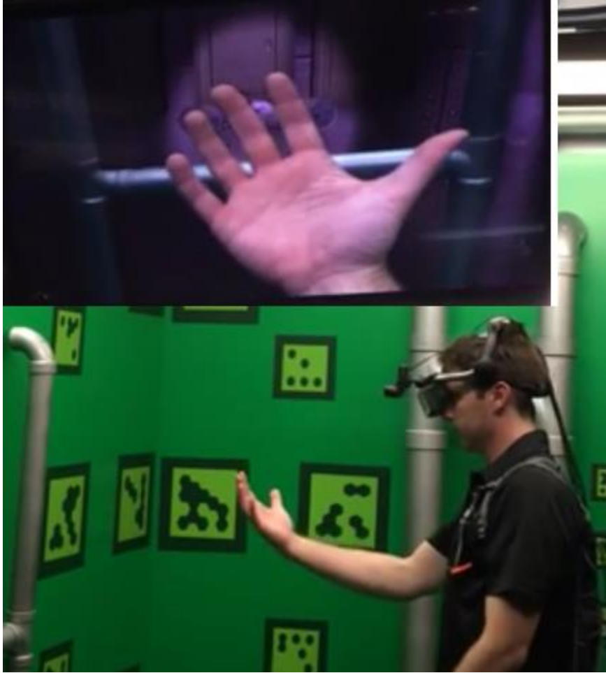
This is a close up of the trainee's hand and the real pipe being displayed over the virtual world (top).
