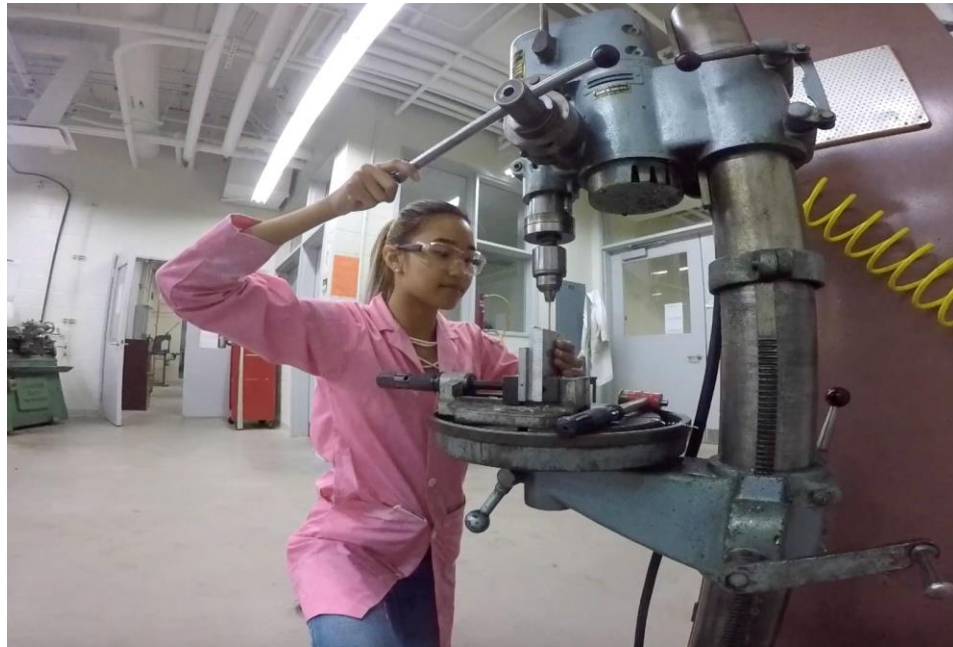
Figure (3) Abby Lacson Machining the holes in Thoracic, Cervical and Lumbar Brackets using a drill press in the maker space in the physics machine shop at the University of Alberta
