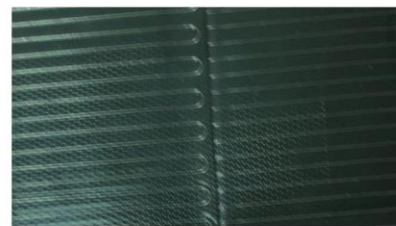
Interaction of light at the air-glass interface for structured glass
