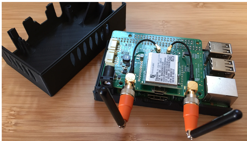
Prototype of an ethernet cellular gateway on a Raspberry Pi with a 3D printed enclosure.
