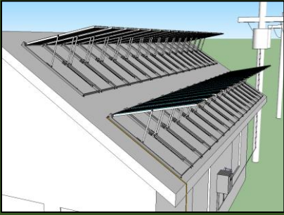
45-degree Longitudinal Solar tracking
