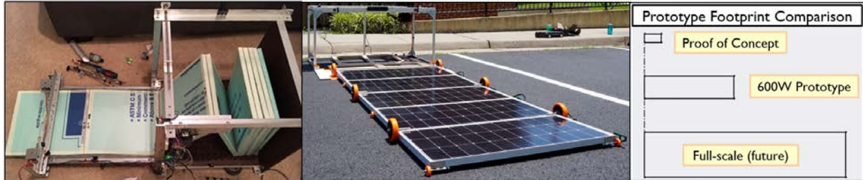
Figure 2: Transition from proof of concept (left) to 600W prototype (middle). (Right) shows the footprint comparison between the proof of concept, 600W, and full scale prototypes
