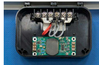
(a) Junction box integration
