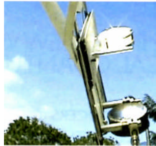
Clear Ceramic collimating lens on test heat exchanger
