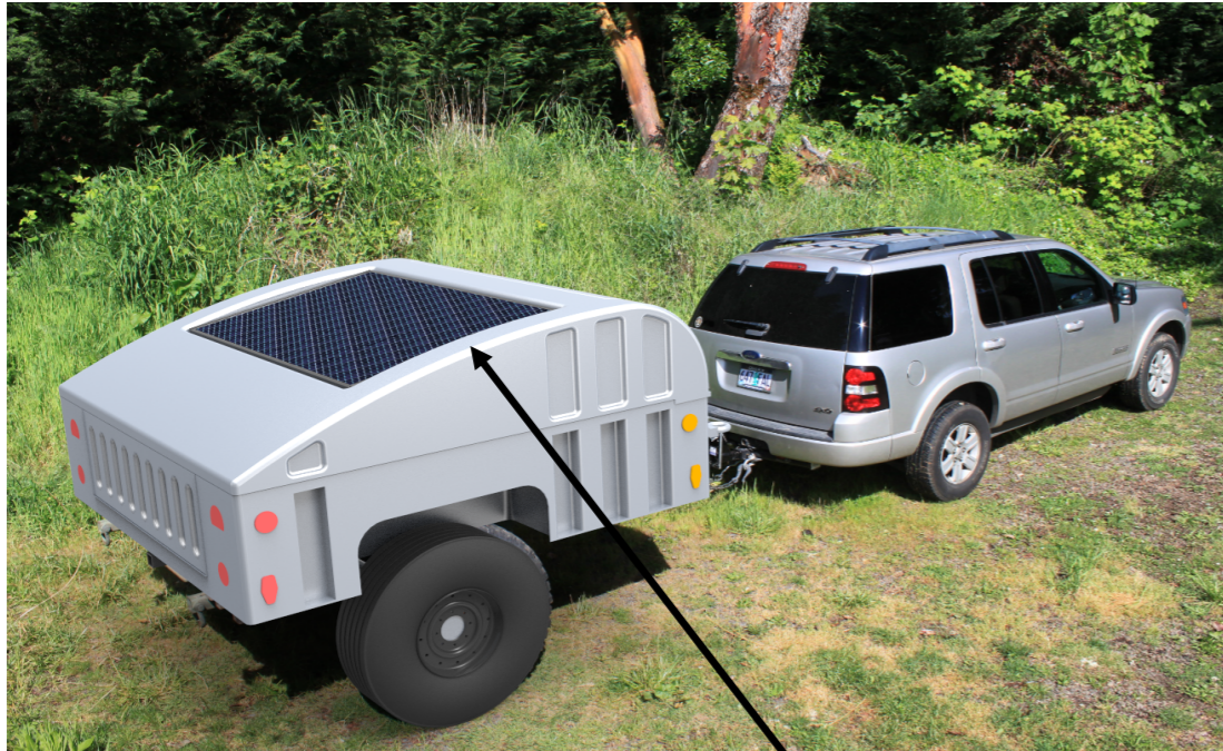
Solar Panels with UV Window
