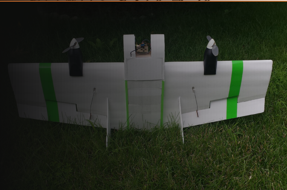
Flex solar integrated into wings enabling continuous operation of system without human intervention
