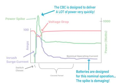
The figure above shows the peak power required to turn on an appliance. The CBC is designed to provide the surge, or spike, so the battery does not have to.
