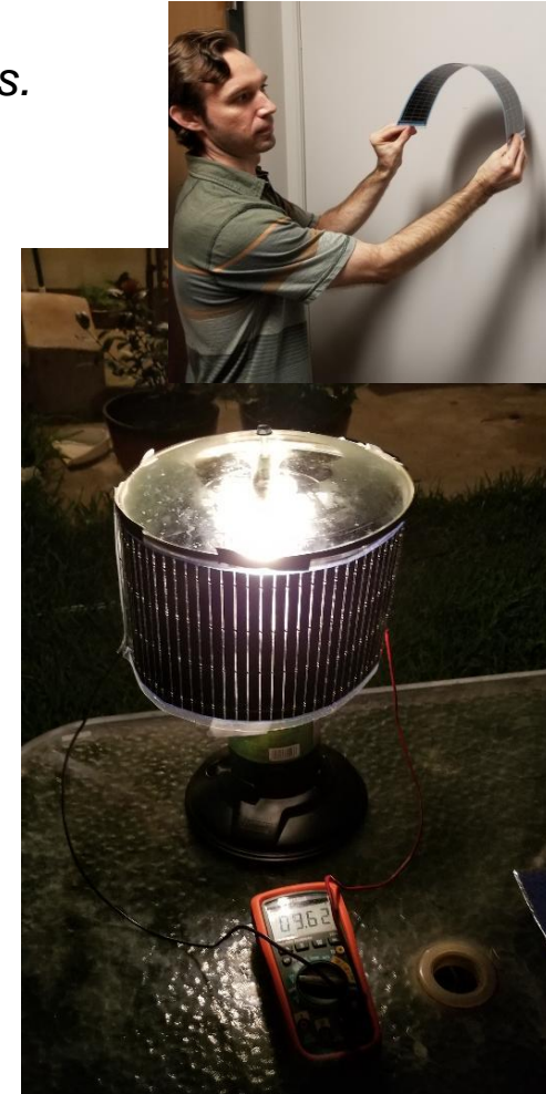
24x7-PV for camping (Functional prototype)
