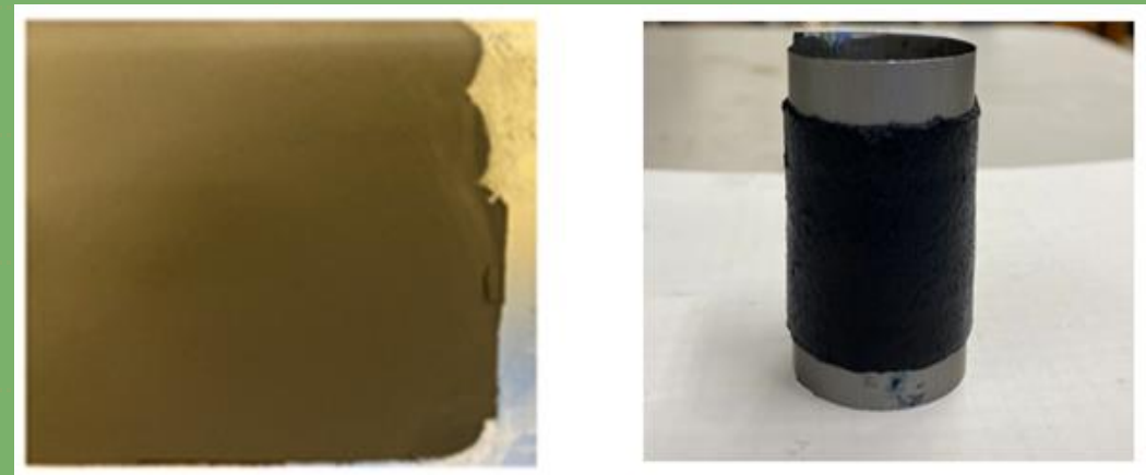
Left: Photo of a casted thick electrode layer (900 \mu\text{m} ) on current collector film using our proprietary method. Right: Cylindrical electrode fabricated using our method with thickness of 1000 \mu\text{m} .
