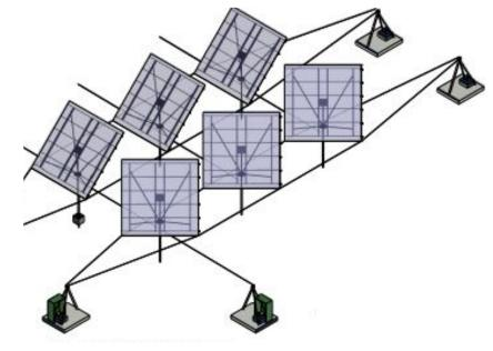
RPV is designed for maximum efficiency. Using winches and cables, the system provides more hours of direct sunlight notably at higher elevations. 14% more energy at a 45 degree latitude can be generated with the RPV solar panel agnostic foundation.
