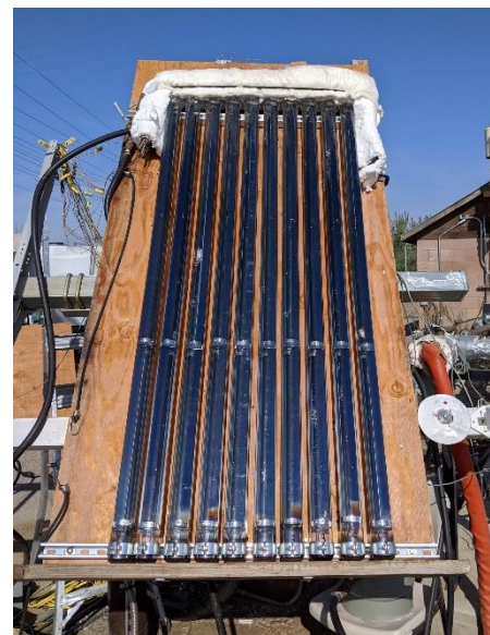
Figure 6 – (left) Experimental solar-to-thermal efficiency. (right) Module under testing.
