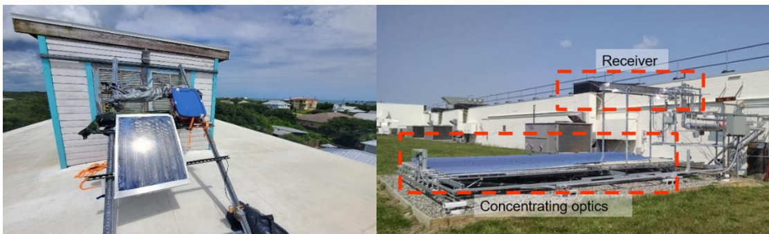
Image 2: (Left) 6 sqft aerogel insulated flat plate collector demonstration. (Right) 19.6 m 2 aerogel-insulated linear Fresnel demonstration.
