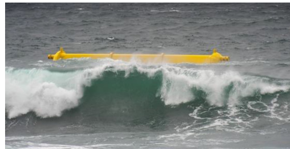
Near-shore device AquaMarine Oyster (a hinged flap)
