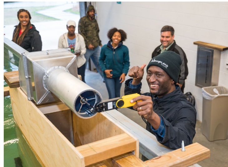
A group of undergraduate students from North Carolina Agricultural and Technical State University experience success testing an oscillating water column wave energy device in the test tank at the Coastal Studies Institute on the East Carolina University Outer Banks Campus. Credit: John McCord, Coastal Studies Institute
